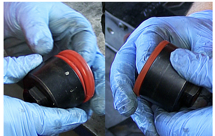
Figure 20. At left, boot bellows protrude from the KT07 sleeve. This will cause damage and improper installation. At right, the bellows are completely tucked into the sleeve and the boot is ready for installation.
