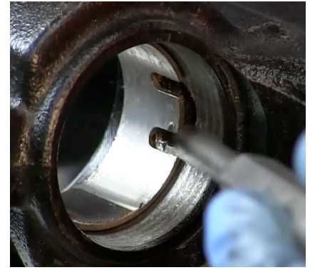
Figure 14. Use punch to bend tab.
