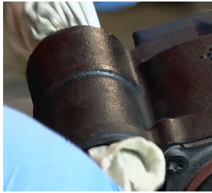
Figure 11. Thoroughly clean bushing cavity.
