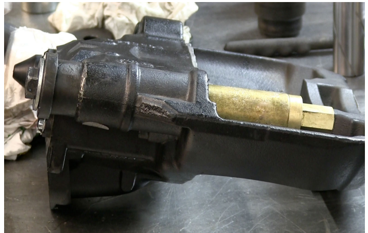
Figure 15. Assemble the Ken Tool components as shown to install the long guide pin bushing.
