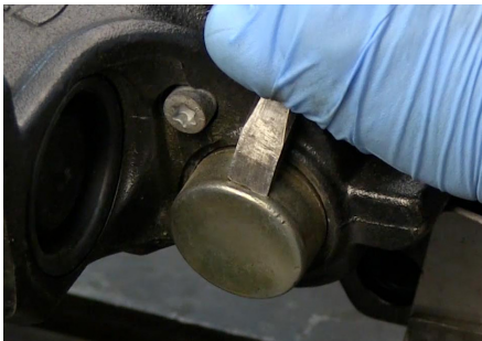
Figure 2. Drive the cap from the edge to help unseat it.
