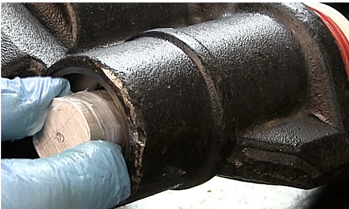
Figure 27. Install the aluminum lubrication directional plug into the long guide pin with the hole facing out.
