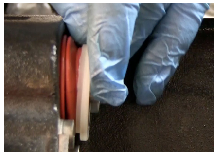
Figure 5. Remove the white retainer rings that seal the boot to the pin.
