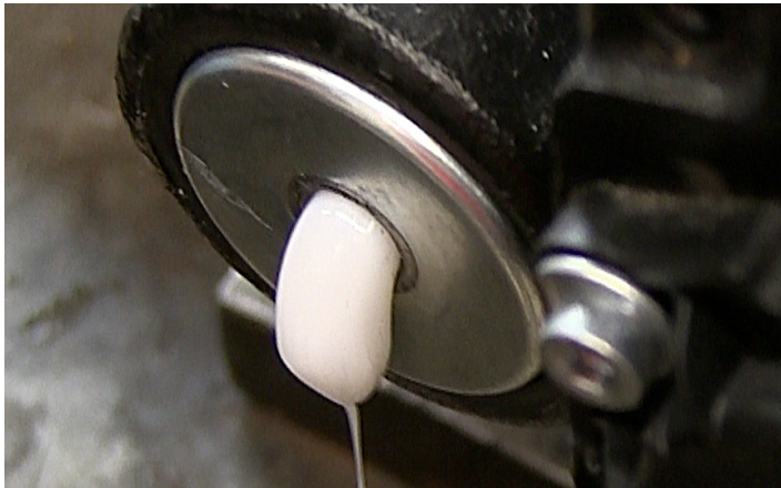
Figure 34. If the caliper was not properly compressed during greasing, you can exhaust excess grease by removing the valve and compressing the caliper.
