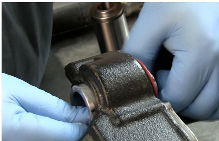
Figure 6. Push the pin from the boot side and extract from the cavity.
