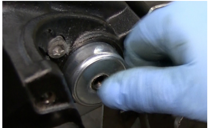
Figure 32. Only the CL-20 kit allows you to drain air from the guide pin boots by removing the valve and using your finger to pump air from the cavity.
