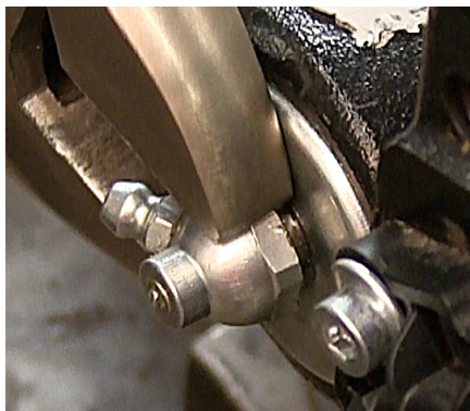
Figure 30. Firmly hand tighten the hydraulic stop valve. Then use a wrench to tighten an additional half turn. Be careful not to over-tighten.
