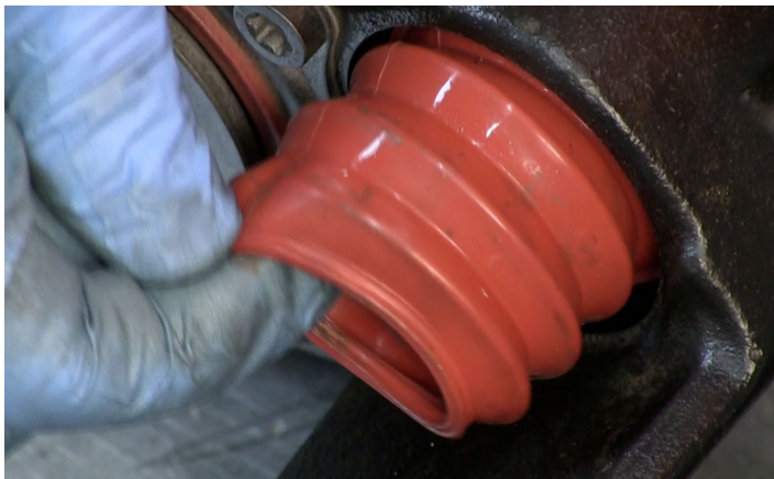
Figure 22. Gently tug on Guide Pin Boots to test seating.
