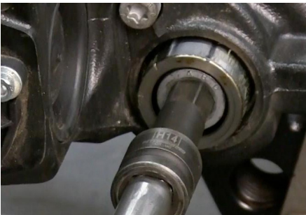
Figure 3. Use 14mm hex bit and impact driver to remove guide pin bolts.
