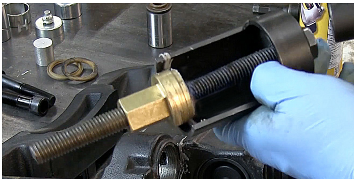
Figure 9. Assemble the Ken Tool components as shown to remove the short guide pin bushing.
