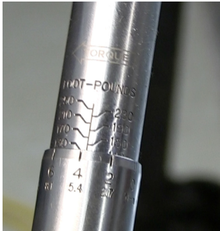
Figure 26. Torque the guide pin bolts to 133 ft-lbs, and add a 90-degree turn.
