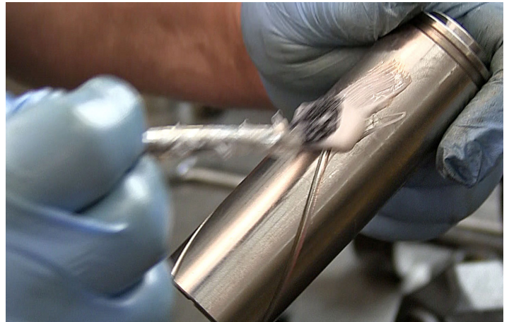
Figure 24. Using a brush, completely fill all Guide Pin grooves with Max-A-Sil 998™ grease.
