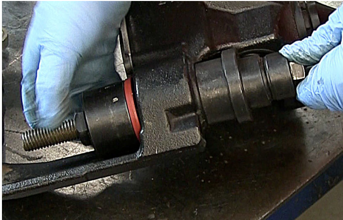
Figure 21. Assembly of Ken Tool components for install of Guide Pin Boots.
