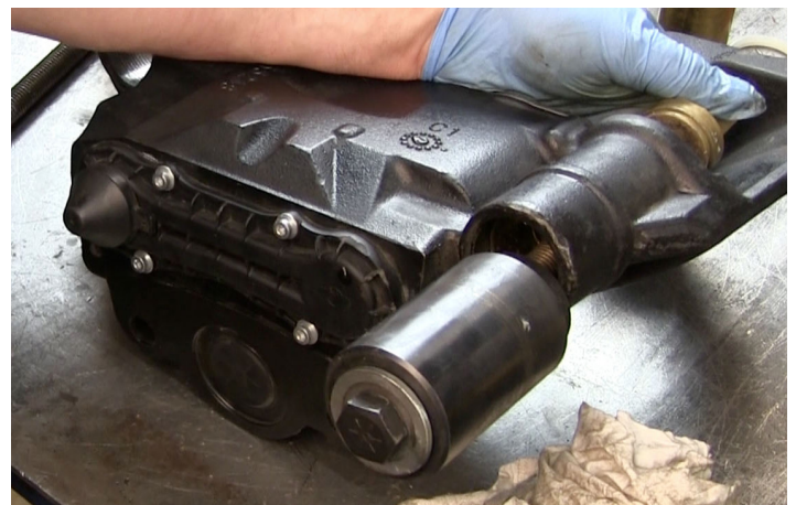
Figure 11. Assemble the Ken Tool components as shown to remove the long guide pin bushing.
