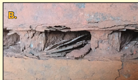
TOP: (A & B) Uncoated rotors leave the ABS ring and vents vulnerable to rusting. This results in ABS sensor faults, and clogged vents that overheat rotors. Such corrosion causes premature replacement of the rotor, and increases maintenance costs.
