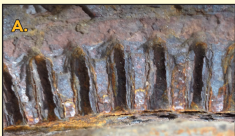
TOP: (A & B) Uncoated rotors leave the ABS ring and vents vulnerable to rusting. This results in ABS sensor faults, and clogged vents that overheat rotors. Such corrosion causes premature replacement of the rotor, and increases maintenance costs.
